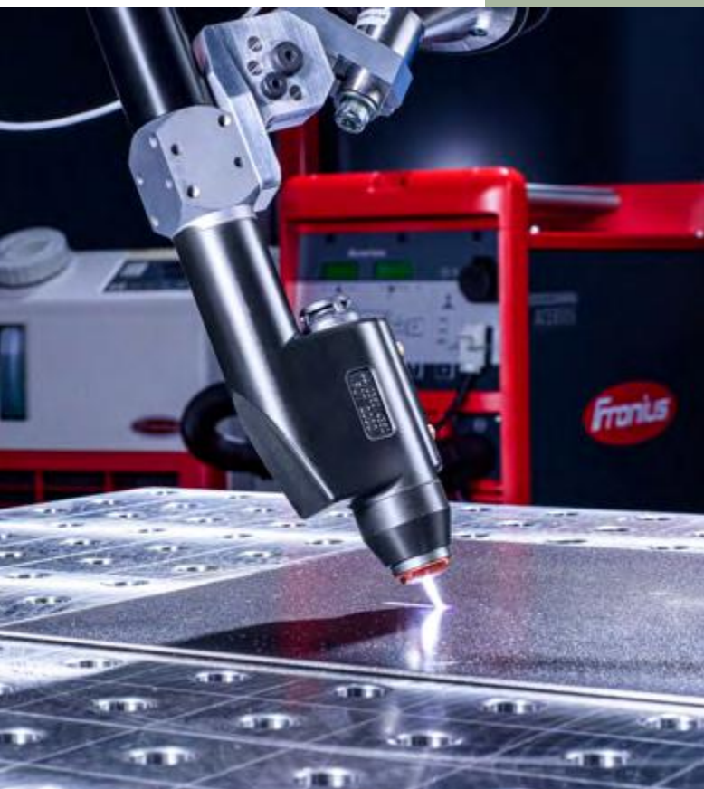
Precision cleaning of material surfaces with the Fronius hot active plasma technology
