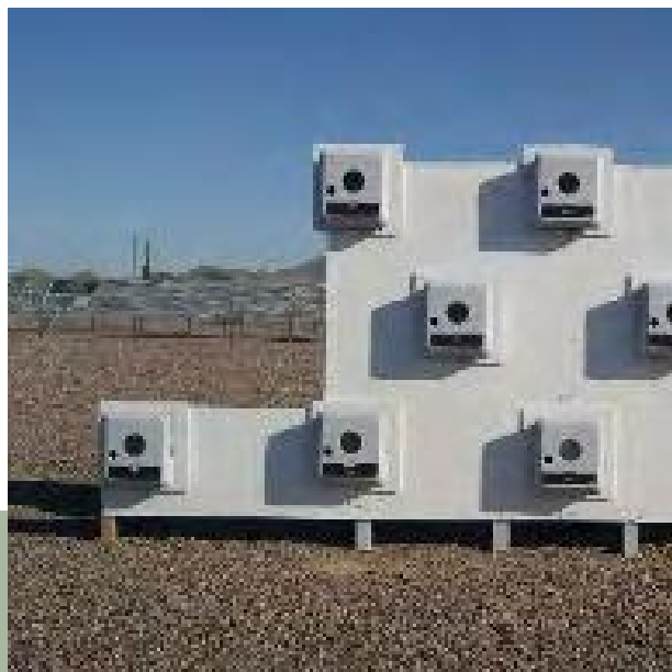
UV resistance tests in Florida and California
