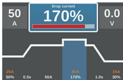
Lowering current I 2 < Main current I 1 | Lowering current I 2 > Main current I 1
