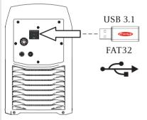
Plug in the supplied Fronius USB thumb drive with FAT32 formatting.
