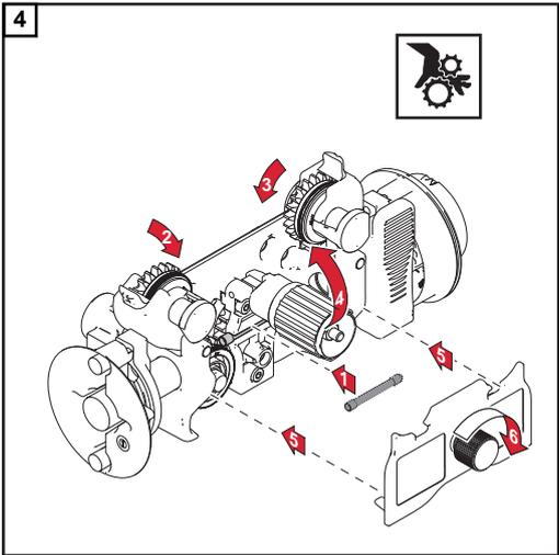
**Inserting the wire spool/basket-type spool**
