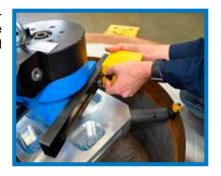
Assemble the ID chuck and install appropriate leg spacers.
