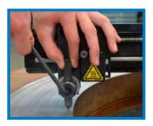
Install the machining arm and slide to desired location.
